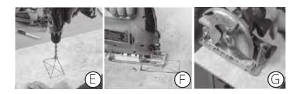
Cut panels for outlets and light switches. Measure and mark the borders where the opening will be with a marker. Drill a 1/2-inch hole using a drill in a corner of the cut-out section (image F). Use a jigsaw to cut the remaining opening, following your tracing (image G).
