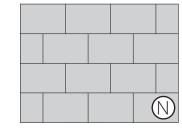
Commonly-used options are running bond (vertical joints are staggered) and stack bond (vertical joints line up).
