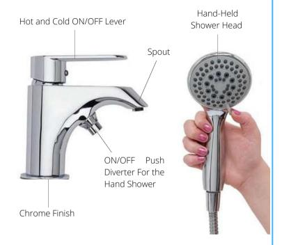
NOTE: This faucet is designed to be installed through 2-1/2" diameter hole for faucet, 1/3" diameter hole for mounting rods, and a 7/8" diagonal hole for the hand shower.
