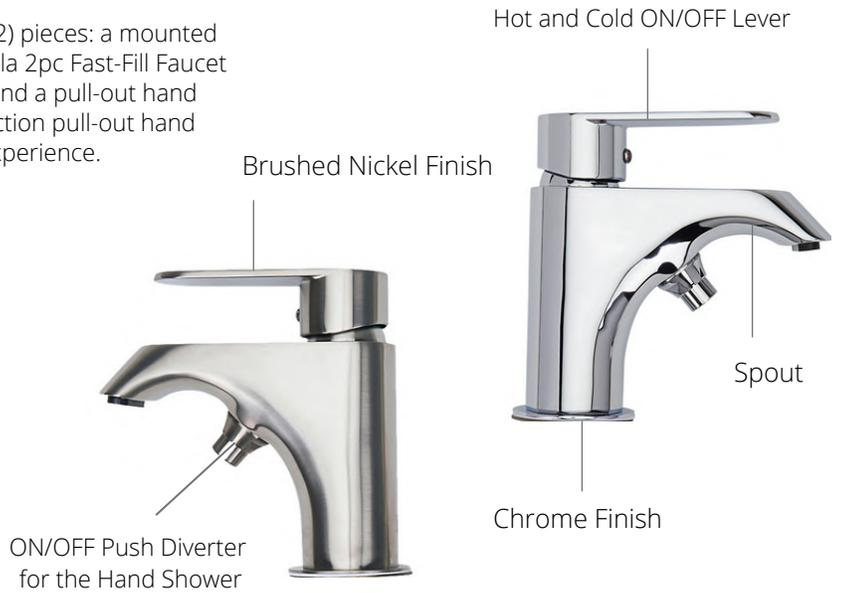
**NOTE: This faucet is designed to be installed through:** G.W: 7.75 kg/ 17 lbs., 2-1/2" diameter hole for faucet, 1/3" diameter hole for mounting rods, 7/8" diagonal hole for hand shower
