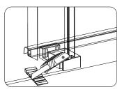
a.Mount anti-jump part 6TB18(2X) on the sliding glass panel to keep distance with 1~2mm to rail profile. b.Cut the extra part of the vertical sealer 6TB04 c.Put top cap 6TB21 onto the wall profile.
