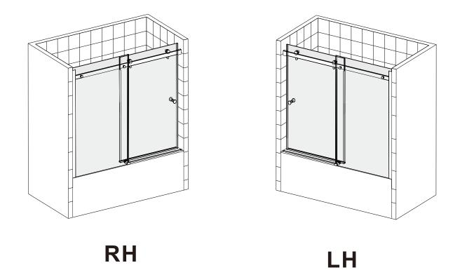
Halo tub door is reversible for Left hand and Right hand. But the mounting instruction is the same for both directions. Below step is followed by Right hand. For left hand, please follow below steps in mirror direction.
