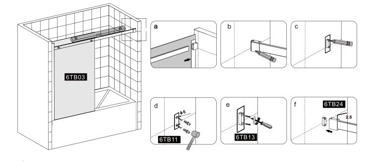
a. Insert the rail profile into wall bracket next to fixed glass panel again. b.Put fixing part H of 6TB19(2X) through the holes of the glass panel to reach rail profile.
