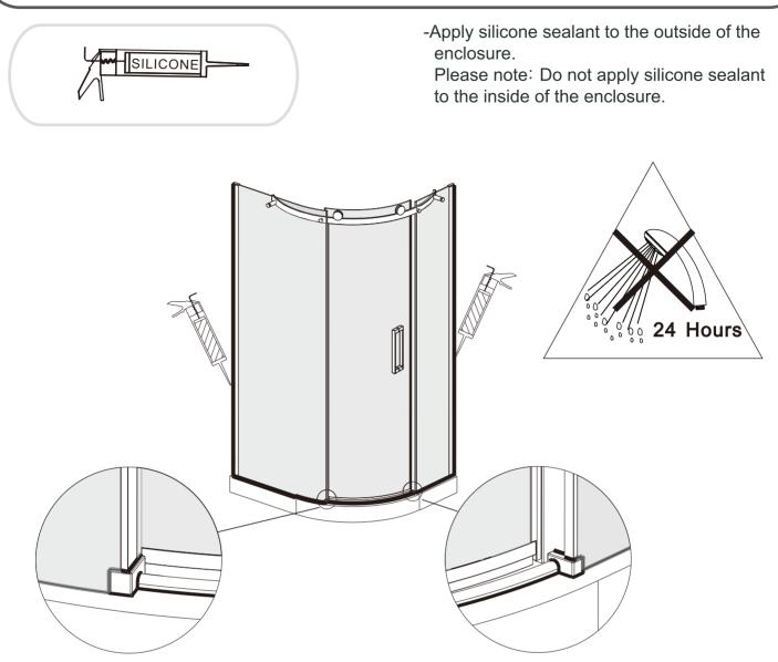
Silicone(according to the thick line position)where the vertical profiles meet the wall, parts meet parts and glass panels meet the tray.
