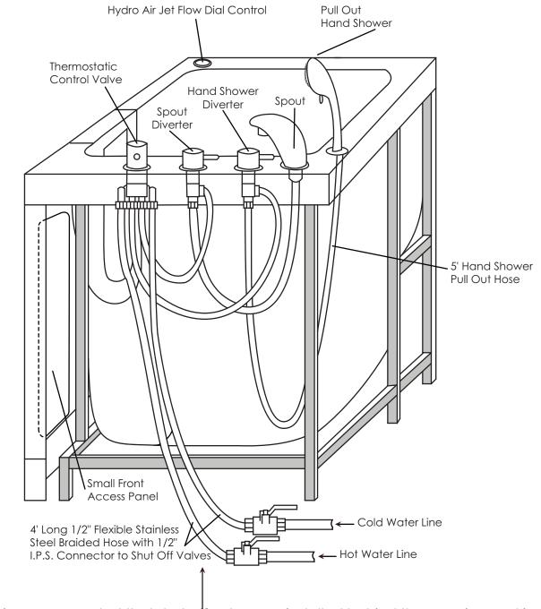
**NOTE:** It is recommended that shut off valves are installed behind the opening and in reach from the small access panel.
