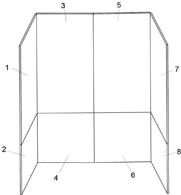
After the shower base is installed please follow the correct sequence of panel installation by referring to its respective drawing.
