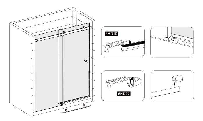
Finally, at all points connected to the wall, the bathtub and the profiles, use silicone sealant only on the outside of the shower enclosure. Please do not take shower within 24 hours after silicon sealant.
